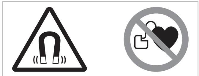
Fig. 9: Warning and prohibition signs on a compressor with permanent magnet motor
