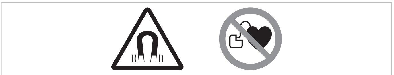
Fig. 15: Warning and prohibition signs on a compressor with LSPM motor
